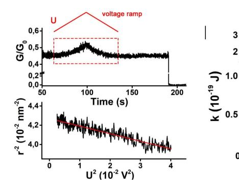
ramp induces a Voltage change of normalized conductance of NT constricted by CF (upper); linear regression of the dependence of  $(r)^{-2}$  on  $U^2$  (lower).
