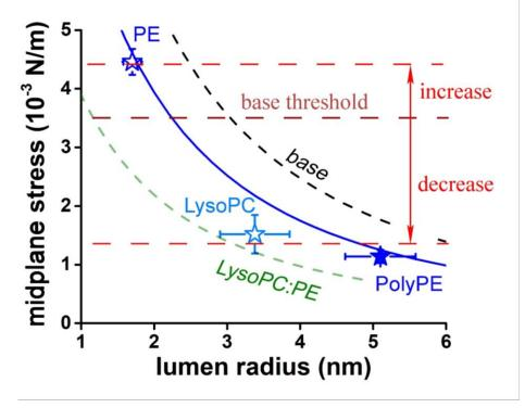
Averaged midplane stress and lumen radius at which structural instability of NT membrane occurs measured for membrane containing LysoPC, DOPE, PolyPE. Curves represent theoretically predicted dependences of midplane stress on lumen radius for the base composition (black), 30 mol% PE or 30 mol% PolyPE containing membrane (blue) and OPC:DOPE 1:1 mixture (olive). Horizontal dashed lines represent the base instability threshold change induced by DOPE (increase) or PolyPE, and LysoPC (decrease).
