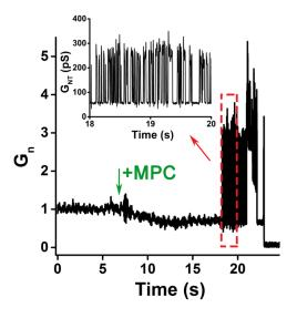
Under similar stress, the presence of conical lipids, such as LysoPC, greatly affects the instability development. MPC induced NT conductnace reduction followed by pores formation in the NT membrane and the NT fission.)
