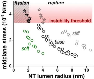
Dependence of NT membrane midplane elastic stress on the NT lumen radius measured for the base (black), stiff (gray), and soft (green) membranes. Fill area indicates elastic stresses lying above the instability threshold at which stochastically structural reorganization of lipid bilayer occurs. Shading marks a region in the stressradius phase space in which the local loss of structural stability of NT's lipid bilayer does not lead to membrane rupture but is resolved by NT membrane fission.
