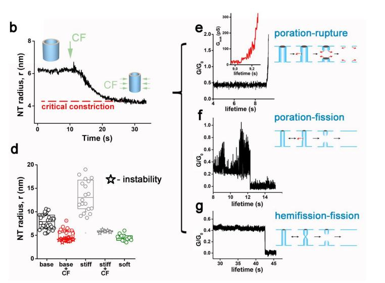
We discriminated three different outcomes of membrane failure to bending stress accumulated in NT pre-fission state: leakless fission, pores formation preceding fission; membrane rupture.
